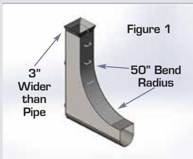
When sizing the boot, be sure the internal width is at least **3" wider** than the outside diameter of the pipe you are installing. In the case of 10" MaxFlex for example, the 11.5" OD would require a minimum internal boot diameter of 14.5". 12" with an OD of 14.5" would need a 17.5" internal boot diameter. The extra width will decrease installation friction on the pipe.
